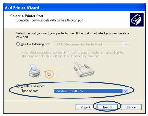
6. Please make sure that the MFP Server and the MFP or Printer have turned on and connected to the network correctly before you continue. Click "Next".
